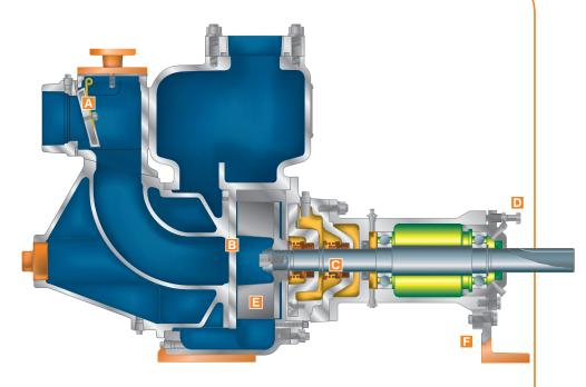
External adjustment saves downtime and extends the life of impeller/wear plate.
