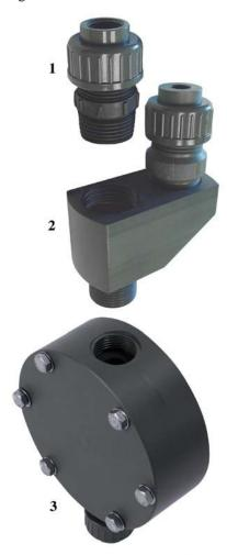
Getting the generated gas out of gas-bearing liquids. The degassing valve (2) fits in between the check valve (1) and the pump head (3), allowing the gas, when generated, to be relieved out and away from the process liquid being transported. Note this arrangement relieves the gas when it occurs, maximizing the fluid transport process.
