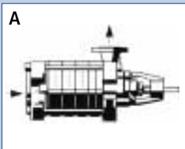
Horizontal baseplate design with axial inlet
