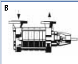
Horizontal baseplate design with radial inlet
