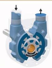
When shaft rotation changes from clockwise to counter-clockwise, the idler carrier (including the idler gear and crescent) automatically rotates 180° through the suction zone to the position shown in the drawing above. This changes the direction of the flow within the pump without changing port positions. On resumption of clockwise rotation, the crescent will swing back to the original position.
